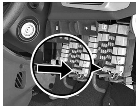
Location of On board diagnostic (OBD II).
