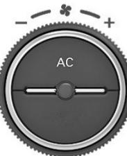
Rotate the knob clockwise to increase & anti-clockwise to decrease the blower speed.
