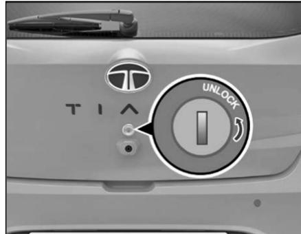
Tailgate can also be opened by using door key. The lock is located on the tail gate.
