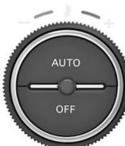
Turning the temperature control knob clockwise increases the temperature of the air. The desired temperature will be increased by steps of 0.5°C. User can select temperature range from 18°C to 30°C. Whereas the anticlockwise direction decreases the temperature.
