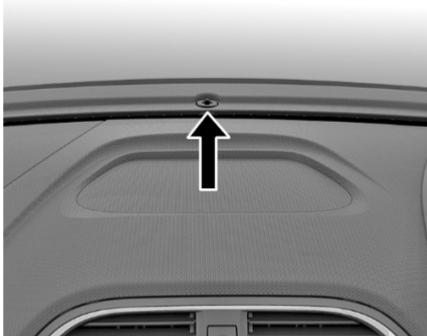
2. In-car sensor on HVAC control panel.
