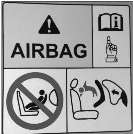
The Airbag Warning Symbol on sun visor reminds of the extreme hazards associated with the use of a rearward-facing child restraint on front passenger seat during airbag deployment. It does not mean that a child cannot occupy front passenger seat and use seat belt. Please refer CRS section for recommended seating position
