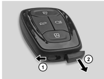
Slide the knob (1) to release the key. Pull the key blade (2) out.
