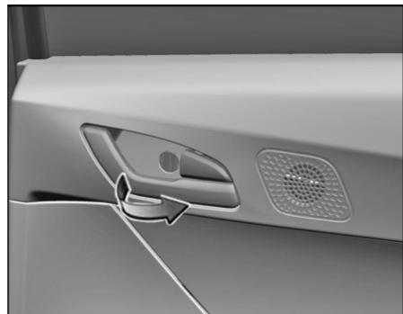
All doors can be opened from inside. To open, pull the door opening lever. All doors can be unlocked by pulling the inside release lever to the intermediate position. When it is further articulated will unlatch the door and can be opened.
