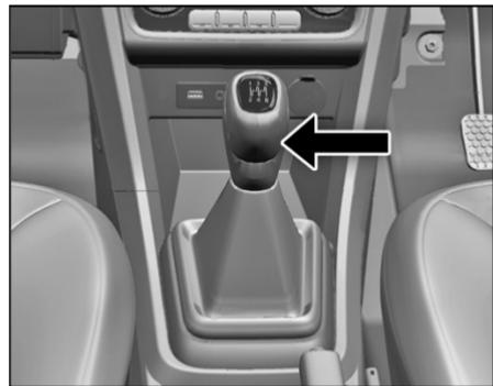
The gearshift pattern is as shown on the gear lever knob. Gear shifting should always be done with the clutch pedal fully pressed.
