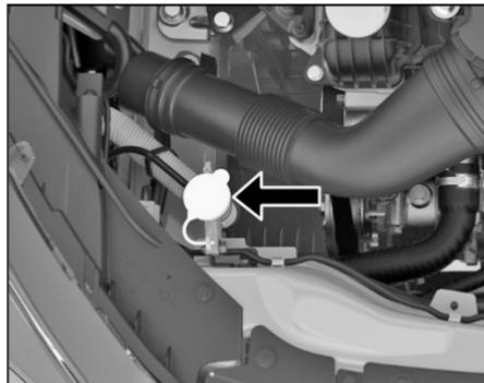
Examine if there is washer fluid in the tank. Fill it if necessary. Use a good quality windshield washer fluid, diluted with water as necessary.
