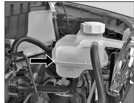
Examine whether the coolant level is between the 'MIN' and 'MAX' marks provided on the coolant reservoir.
