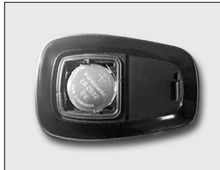
2. Replace with new battery in the smart key battery slot.
