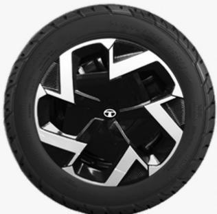
Insert a piece of cloth between the spokes of the wheel cover and pull it outwards. Take out detached wheel cover from the wheel rim.
