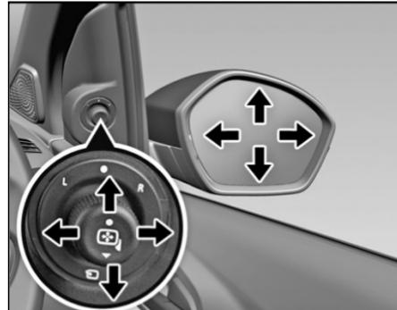
To fold / unfold the ORVMs, keep the Selector switch in center position (i.e. neither 'L' nor 'R' position) and then toggle down. This will operate when the ignition switch is in the "ACC" or "ON" position.
