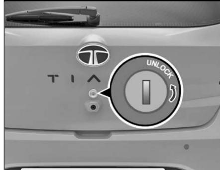
Tailgate can also be opened by using door key. The lock is located on the tail gate. For closing, pull the tail gate down and close it with a slight swing.
