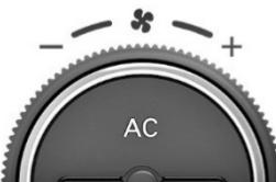
Press the AC compressor ON/OFF button to turn the air conditioning ON or OFF. The AC icon shall be activated on the display when the AC is ON.
