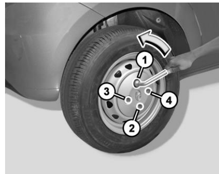
Wheel nut removal
