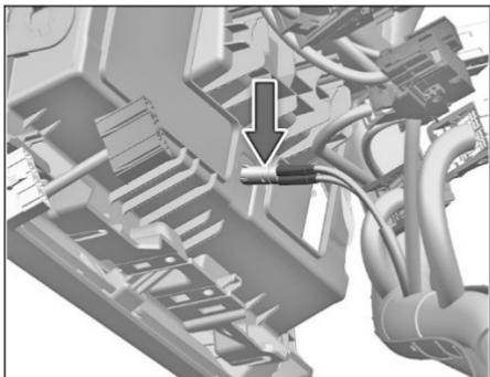
6. Pull out the fuse from fuse box modules from available cutout as shown below.
