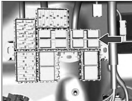
7. Check the fuse of required function with help of fuse box sticker present at shown location.
