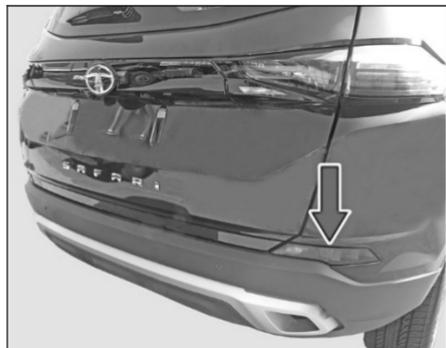
For switching 'ON' the rear fog lamps, front fog lamp must be 'ON'.
