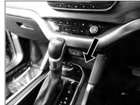
Place for keeping wallet / mobile is provided in front of Gear shifter lever.
