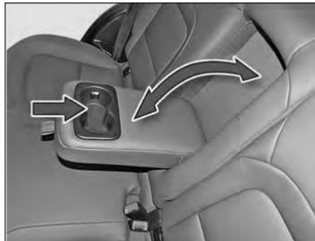
A foldable arm rest has been provided in the rear seat. It also has two cup holders, which can be accessed by opening the cover. When not required, fold the armrest back into the seat.
