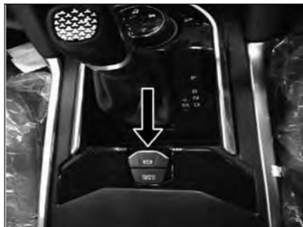
AVH will be released when accelerator pedal is depressed in first gear or Reverse gear (in case of Manual Transmission) and R (Reverse), D (Drive) or Manual shift mode (in case of Automatic Transmission).
