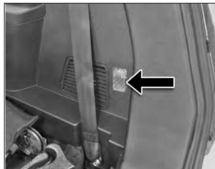
Boot lamp is available in the rear luggage compartment to light up the luggage area. Boot lamp is without switch type. It will be ON only when tailgate is open.
