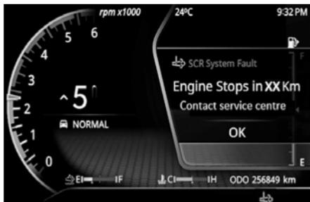
If the vehicle is run without rectifying the SCR system (through TATA MOTORS service center), warning message will continue with corresponding distance gradually reducing to 0 km.
