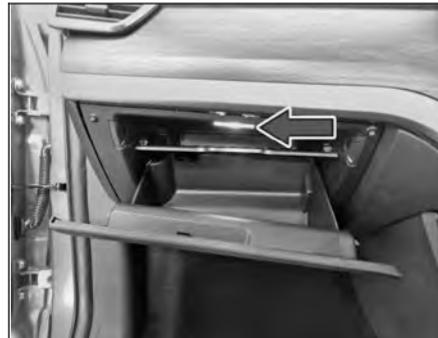
The glove box lamp illuminates when the glove box is opened.
