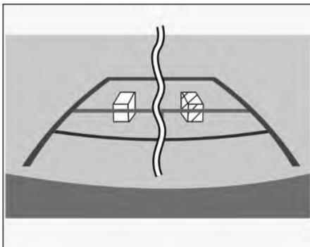
The distance guidelines will appear to be closer to the vehicle than the actual distance.
