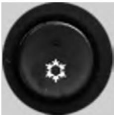
Press the switch to activate / deactivate the AC. The indicator lamp in the button will light up when climate control is activated.
