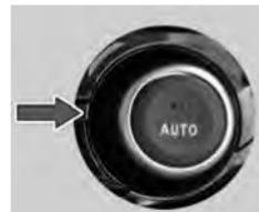
Turning the temperature control knob clockwise increases the temperature of the air. The desired temperature will be increased by steps of 0.5°C. User can select temperature range from 18°C to 30°C. Whereas the anti-clockwise direction decreases the temperature.
