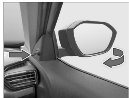
You can adjust the outer rear view mirrors manually by joy stick knob located in the driver and front passenger door panel.
