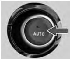
To put the automatic climate control in fully automatic mode:
