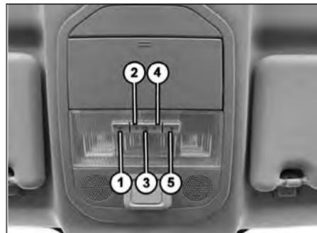
1. Spot / Reading Lamp for Front passenger side
