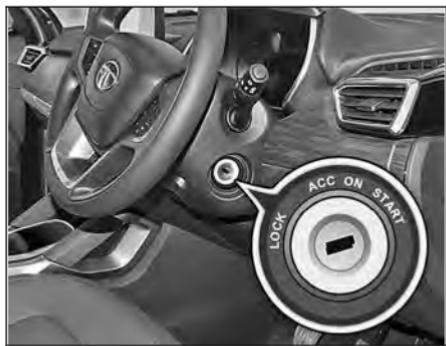
The ignition switch has the following four positions:
