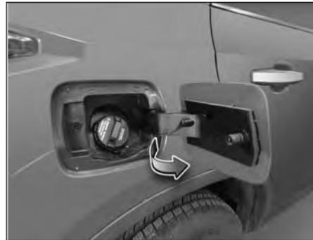
3. To open the fuel cap by turning it in counter clockwise for fuel filling.
