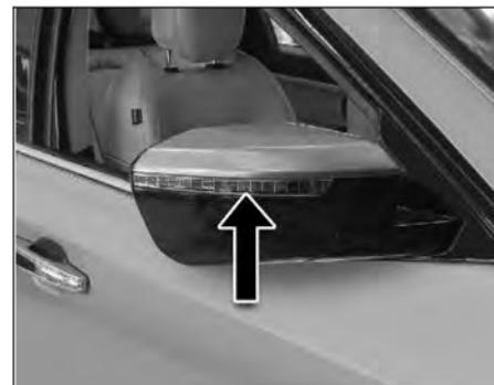
It is provided on outer part of ORVM. It will turn ON when the turn signal indicator switch is ON and Hazard Warning indicator switch is ON.
