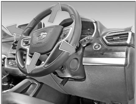
4. Push release lever up completely to lock the steering column.
