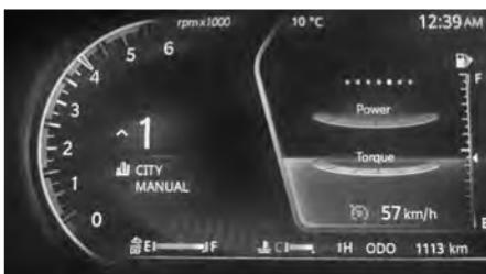
Indicates the amount of power and torque delivered by engine in the particular driving condition.
