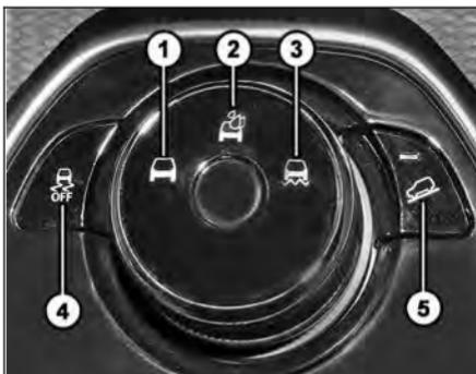
Rotate the knob clockwise to select the terrain mode.
