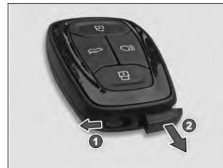
Slide the knob (1) to unlatch the key. Pull the key blade (2) out.
