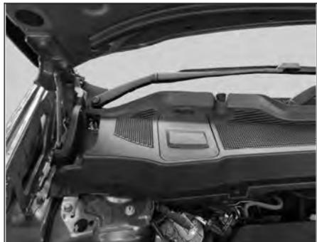
Pull the notch and release the top cover.
