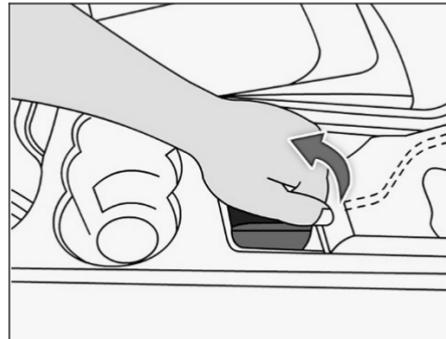
To apply the parking brake, hold the lever as shown in above figure with knuckle facing towards vehicle front and pull the lever.
