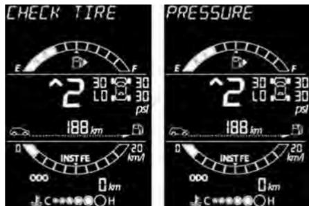
TPMS screen with combination of failures in tires
