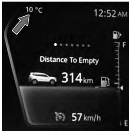
This displays outside ambient temperature in units of °C with the resolution of 1 °C.
