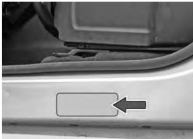
VIN plate near Front passenger seat (LHS outer side)
