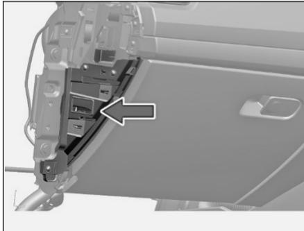
3. Open glove box and remove complete assembly by removing highlighted 4 screws.
