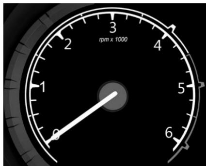
Tachometer indicates engine speed in revolutions per min (rpm).
