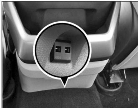
Smart charger (dual) is available be-tween the front passenger seats below the rear stowage area for second row passengers.
