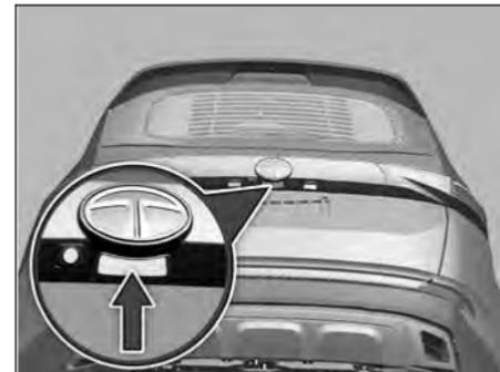
If vehicle is locked and tail gate is closed. Tail gate switch is pressed with valid smart key in the authentication range, Tail gate gets unlatched.
