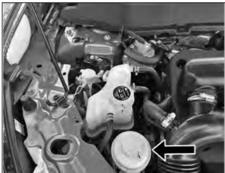
The level of the power steering fluid should be between the MIN. and MAX. mark on the side of the power steering fluid container. If the level falls below the MIN. mark, add recommended fluid.
