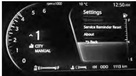
To change the option from unit to service reminder reset by pressing on the RHS of steering switch.
