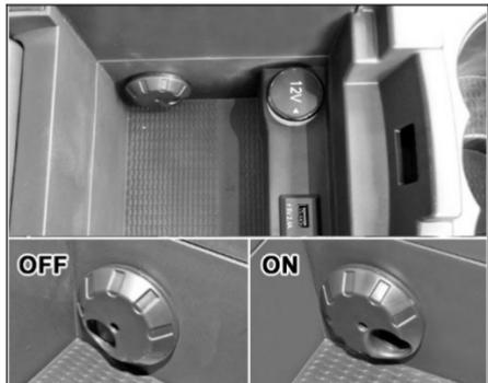
On selected models cooling facility is provided below driver foldable arm rest. It cools only when the A/C is ON. Close the vent by rotating the knob, whenever cooling is not required.
