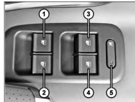
1. Front Window Winding Switch (Right)
