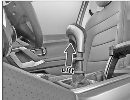
For engaging reverse gear, lift the latch and by keeping latch lifted, shift to reverse position.
