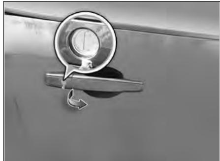
Insert the key and turn it clockwise to lock and anticlockwise to unlock the door.
