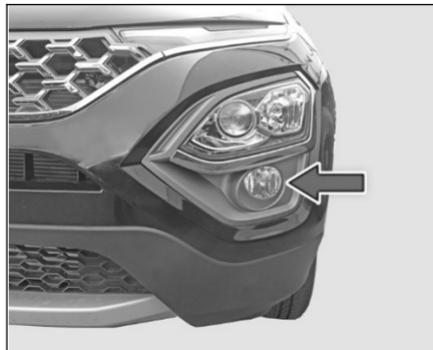
For switching 'ON' the Fog lamps, either the Head Lamp or Parking lamp must be 'ON'.
