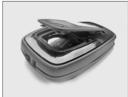
2. Replace with new battery in the smart key battery slot with proper polarity of battery.
