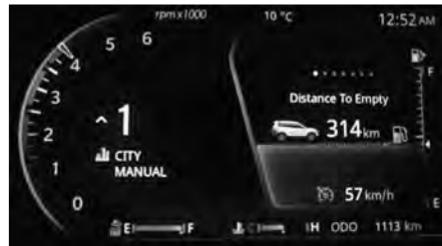
The above DTE screen indicates approximate distance in 'km' that your vehicle can travel with available fuel in the tank.
