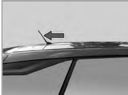
Antenna is located on the roof. Turn antenna anticlockwise to remove from vehicle, if required.
