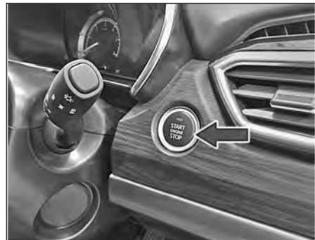
Start/Stop switch is provided on the dashboard towards the right side of steering wheel.
