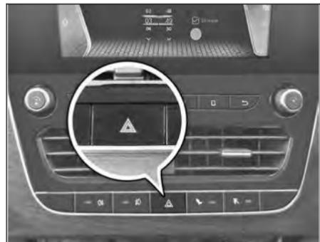
Press the hazard warning switch to activate the hazard warning. All the turn signal lamps will flash simultaneously. To turn OFF, press the switch again.
