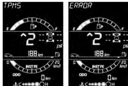
TPMS screen with leakage
