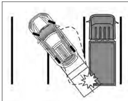
Visually check the surroundings and the area behind the vehicle. In the case shown below, the truck appears to be outside of the vehicle width guidelines and the vehicle does not look as if it hits the truck. However, the rear body of the truck may actually cross over the vehicle width guidelines. In reality if you back up as guided by the vehicle width guidelines, the vehicle may hit the truck.
