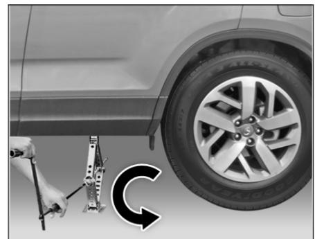
Remove wheel mounting nuts with the help of wheel spanner and take out flat tyre.
