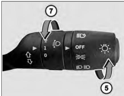
Inner rotary switch on right hand stalk is provided for head lamp leveling. With the inner rotary switch, Head lamp leveling can be done with head lamp in Low Beam and in 'ON' position. Select correct position before start of trip when the vehicle is stationary. Depending on the number of passengers and luggage in the vehicle headlamp focus may change. This can be adjusted by rotating the knob to one of the 3 level positions.
