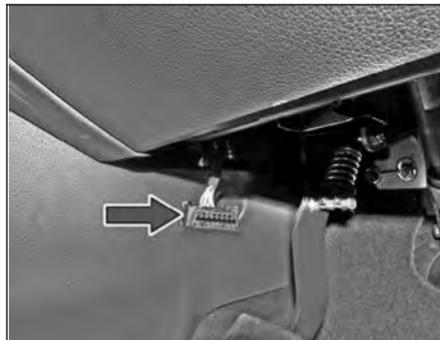
On board Diagnostics or OBD, is an automotive term referring to a vehicle's self-diagnostic and reporting capability. The OBD system allows continuous diagnosis of the components of the vehicle correlated with emissions. This system warns the driver, by turning "ON" the Malfunction Indication lamp (MIL) on the instrument cluster, when a fault causes emission levels to increase.
