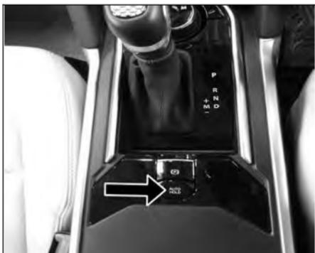
The system eliminates the requirement of depressing the brake pedal continuously when the vehicle stops in between running.
