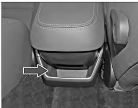
Stowage for rear passenger is provided on rear side of floor console between the front passenger seats. It can be used to keep mobile charger, mobile and small items like wallet, Power bank etc.
