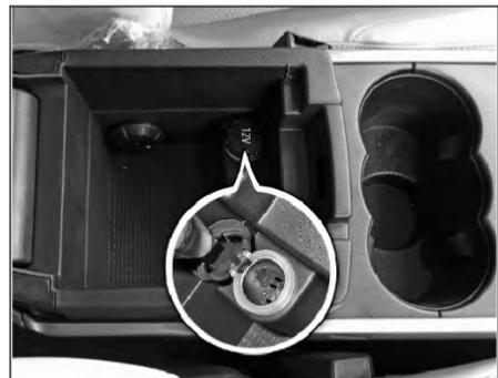
Power socket is available inside the cooled storage box on the center console. The power socket will work when the ignition switch is in the "ACC" or "ON" position. This socket can be used to provide 12V (10A) power for electrical accessories.
