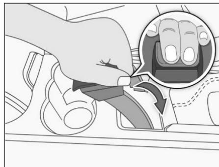
To release parking brake, hold the lever and pull the lever up slightly, press the knob with the help of middle and ring finger as shown in figure and release the parking brake.
