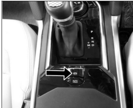
APB switch is located behind the gear shift lever replacing the conventional parking brake (Hand brake lever connected to brake mechanism by cable). APB is applied by pulling up the APB switch and can be released by pushing down the APB switch which needs the vehicle to be at ig-
