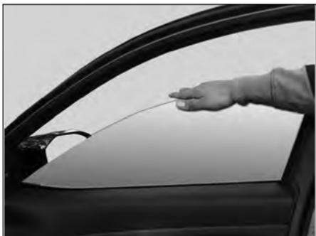
The Anti-pinch module is provided. It will stop window upward movement if any ob-
