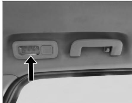
Side reading lamps (applicable for variants with Sunroof) are provided above second row seat passenger doors.
