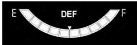
The Indicator should be within the acceptable range. i.e., between “E” and “F”. When DEF in tank is near to empty position, DEF tell tale near to gauge will glow with subsequent text messages on LCD screen. To change screen over from IFE to DEF Gauge press mode button. If DEF level reaches to critically low level, only DEF gauge will be displayed. Screen will
