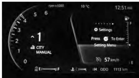
You can enter into setting screen by pressing select button while being in setting screen.
