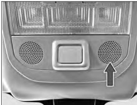
Mics are provided on roof near the roof lamp.
