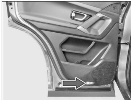
Puddle / Ajar Lamp is provided on driver, front passenger & rear doors trim. It will be ON only when particular door is in open condition.
