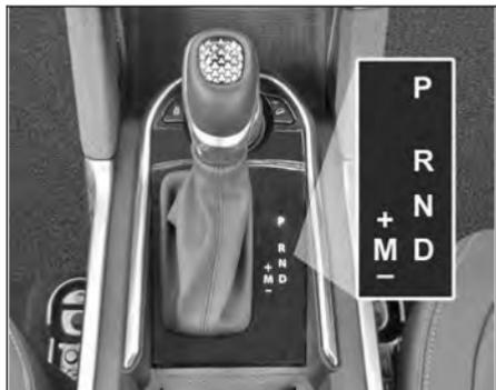
The Automatic transmission has 6 forward and one reverse gear. The individual gears are selected automatically, depending on position of gear shift lever.
