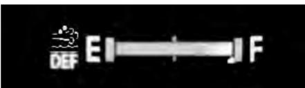
The Indicator should be within the acceptable range. i.e., between "E" and "F". When DEF in tank is near to empty position, DEF telltale near to gauge will glow with subsequent Text alert on DIS Screen. If DEF level reaches to critically low level, then DEF Gauge will be replaced by the permanent text alert along with buzzer.
