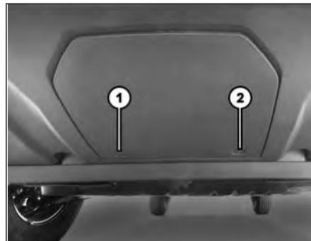
For removal of cover, pull the rear side down.
