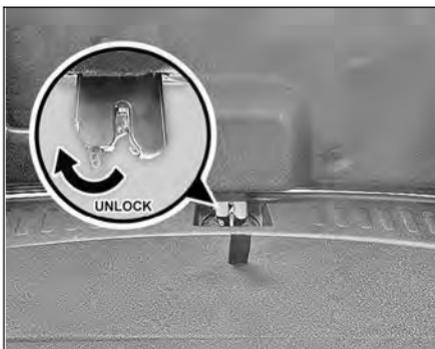
In emergency situation like key or vehicle battery is discharged or electrical malfunctioning, you can unlock the tailgate from inside as per procedure given below:
