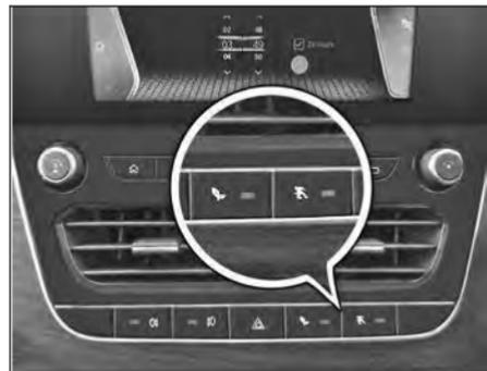
Drive mode selection switches are provided on center console for activation. Press the switch to select the mode.
