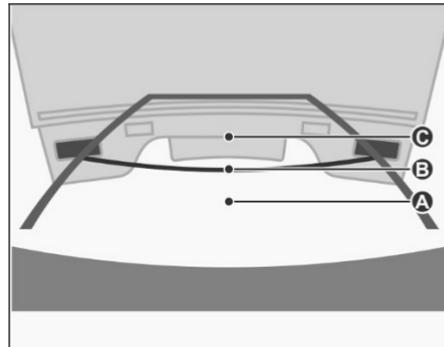
Visually check the surroundings and the area behind the vehicle. On the screen, it appears that a truck is parked at point B. However, in reality if you back up to point A, you will hit the truck. On the screen, it appears that A is closest and C is furthest away. However, in reality, the distance to A and C is the same, and B is farther than A and C.
