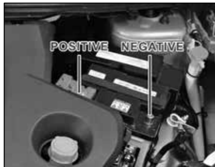
Battery location- Diesel
