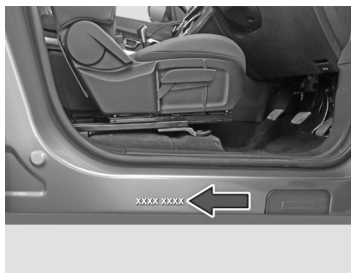
Chassis No. punching near driver seat (RHS outer side)
