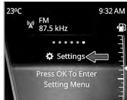
User can enter into setting by pressing select button **②** while being in setting screen.
