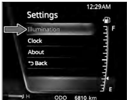
To change the option by pressing **< >** button on RHS of the steering wheel.
