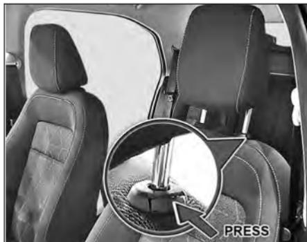
Adjust the head restraint so that it is as close to the head as possible and the center of the head restraint supports the back of the head at eye level. This will reduce the risk of injury to the head and neck in the event of an accident or similar situation.
