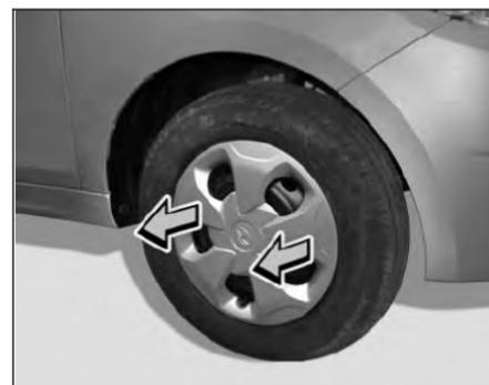
Insert a piece of cloth between the spokes of the wheel cover and pull it outwards.
