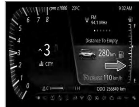
When fuel in the tank nears empty, low fuel warning tell-tale light glows. Fill fuel as soon as possible.
