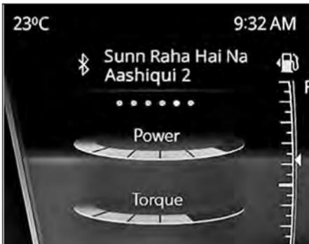
Indicates the value of Power and Torque delivered by engine in the particular driving condition.
