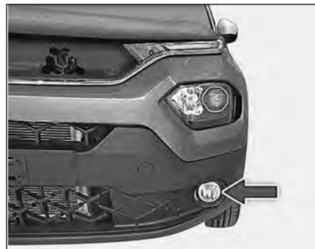
The front fog lamps are located on the front bumper. In poor visibility conditions due to fog, snow or rain, the fog lamps make visibility better and make it easier for other road users to see you. It turns to 'ON' when the fog lamp switch is turned on when the ignition is 'ON' and when the position and parking/ head lamp is 'ON'. An indicator on the instrument cluster will come on when the front fog light is 'ON'.
