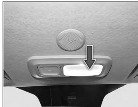
**ON** - The lamp will turn 'ON' as long as the switch is in this position.
