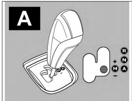
Auto mode will be engaged only when vehicle is stationary and brake pedal pressed. An audio signal indicates when Automatic gear is engaged. **A** will be indicated in instrument cluster.
