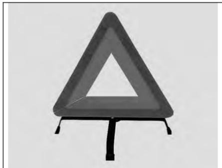
Use advance warning triangle to warn the approaching traffic in case of vehicle break-down or during emergency, where your vehicle could become a potential traffic hazard.
