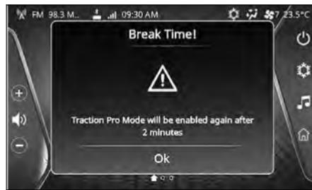
If the terrain is beyond physical limit of the Traction Pro Mode, notification pop up as described in below image will be displayed on the infotainment system. Please take external aid to tow the car in this situation.
