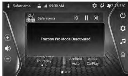
In case there is any system temperature high is identified during the operation of Traction Pro Mode, Traction Pro Mode will be disabled temporarily for around 2 minutes.
