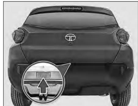
If the vehicle is locked, tail gate is closed and tail gate DHS switch is pressed with valid smart key in the authentication range the tail gate gets unlatched.
