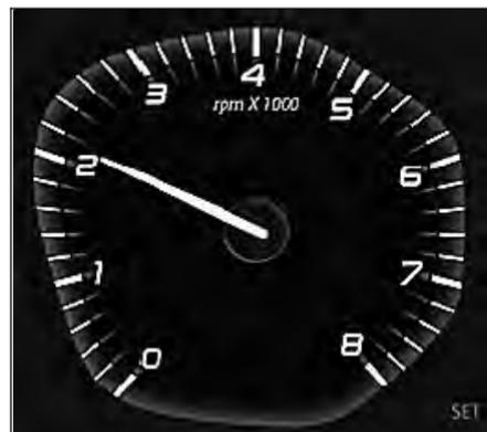
Tachometer indicates engine speed in revolutions per min (rpm).
