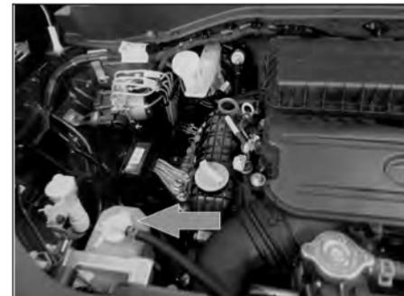
Examine whether the coolant level is between the 'MIN' and 'MAX' marks provided on the coolant reservoir.
