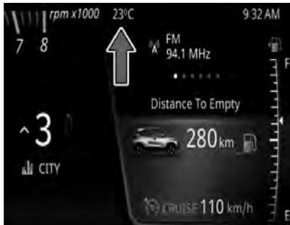
This displays outside ambient temperature reading with an accuracy of  $\pm 1^{\circ}\text{C}$ .
