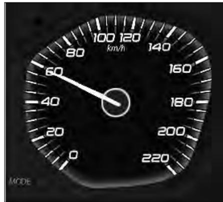
Speedometer indicates the vehicle speed in kmph.
