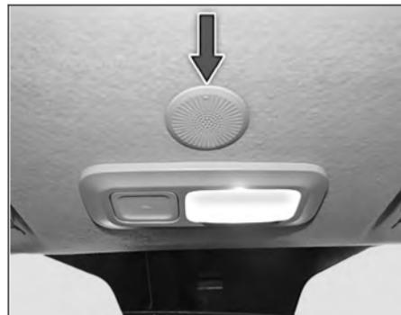
Mic is provided near the roof lamp.
