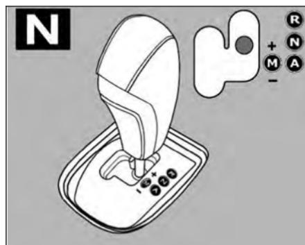
Vehicle is in neutral gear position. This will be indicated **N** on instrument cluster.
