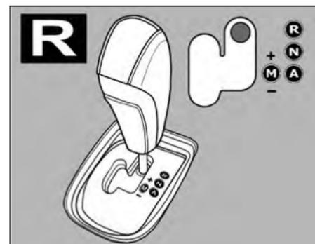
Reverse gear will be engaged only when vehicle is stationary and brake pedal pressed. An audio signal indicates when reverse gear is engaged. **R** will be indicated on instrument cluster.
