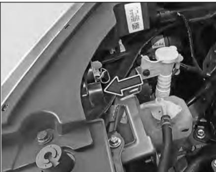
2. Remove the Bulb Access cover by rotating as per the direction arrow shown on the cover.
