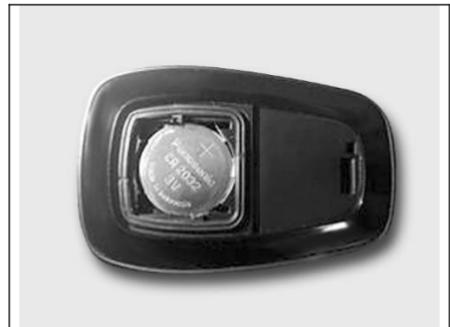
2. Replace with new battery in the smart key battery slot.
