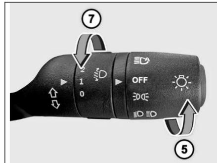
Inner rotary switch on right hand stalk is provided for head lamp leveling. With the inner rotary switch, Head lamp leveling can be done with head lamp in Low Beam and in 'ON' position. Select correct position before start of trip, when the vehicle is stationary. Depending on the number of passengers and luggage in the vehicle headlamp focus may change. This can be adjusted by rotating the knob to one of the three level positions.
