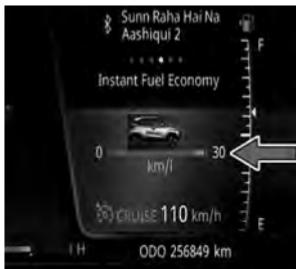
To reach the Instant Fuel Economy in the Instrument cluster. Press the **< >** button on the RHS of the steering wheel.
