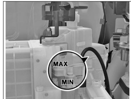
The level of the AMT oil reservoir level should be between the 'MIN' and 'MAX' marks on the side of the container. If the level falls below the 'MIN' mark, add recommended oil.
