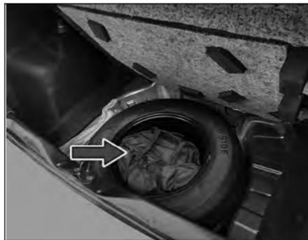
Tool kit and Jack are accommodated in Tool kit bag located in the rear boot.
