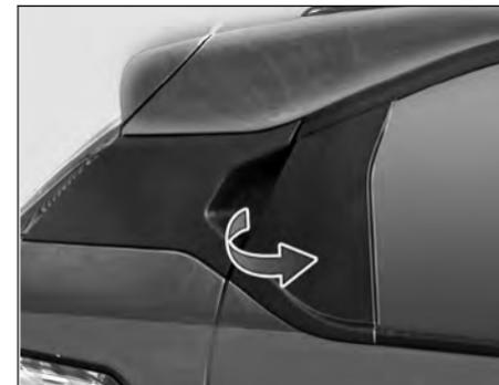
To open the door, press the lever provided inside the handle and pull.
