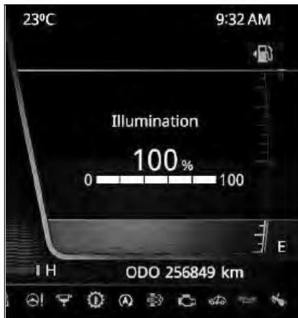
To increase the illumination from 20% to 100% in five steps by pressing **>** button on RHS of the steering wheel.
