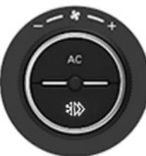
This helps cabin to reach to comfort temperatures quickly by optimally setting the air conditioning to maximum cooling. Also, if required, the driver window will roll down to flush the hot air from inside the cabin. XPRESS Cooling can be turned On/Off by XPRESS COOL knob on FATC panel or by a soft key from Head Unit.
