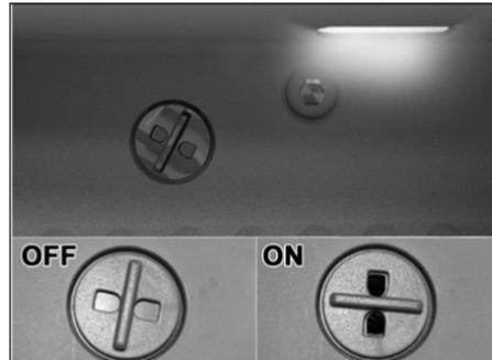
On selected models glove box is provided with a cooling facility. It cools the glove box only when the front A/C is ON. Shut OFF the vent by rotating the knob, whenever cooling is not required.
