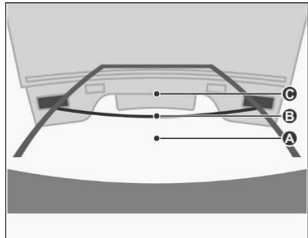
Visually check the surroundings and the area behind the vehicle. On the screen, it appears that a truck is parked at point B. However, in reality if you back up to point A, you will hit the truck. On the screen, it appears that A is closest and C is furthest away. However, in reality, the distance to A and C is the same, and B is further away from A and C.
