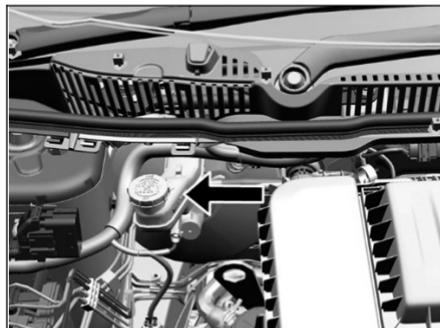
*Brake Fluid Level (Diesel)*
