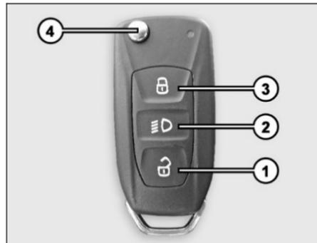
This feature helps to find and reach the parked vehicle or to reach home in dark/cloudy condition after parking. Red LED will be flash on the remote. To switch 'OFF' the approach lights, press and release the same button or it automatically turns 'OFF' after certain time.
