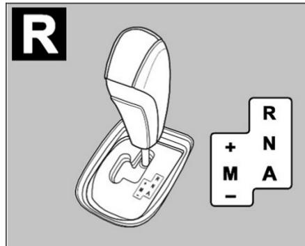
Reverse gear will be engaged only when vehicle is stationary and brake pedal pressed. An audio signal indicates when reverse gear is engaged. **R** will be indicated on instrument cluster.
