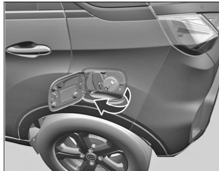
For closing, turn the fuel cap clockwise and gently push the fuel flap till it gets locked.
