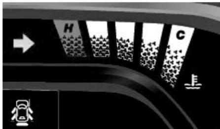
When the ignition switch is in the "ON" position, this gauge indicates the engine coolant temperature. The indicator should be within the normal, acceptable temperature range i.e. between "H" and "C". If the indicator approaches "H", overheating is indicated by a RED bar.
