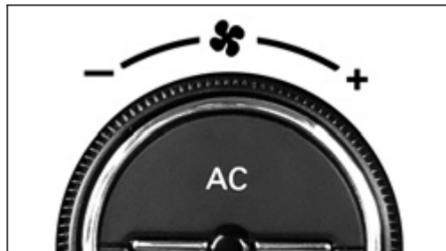
Press the AC ON/OFF button to turn the air conditioning ON or OFF. The AC icon activated on the display when the AC is ON.
