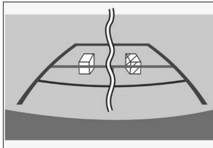
The distance guidelines will appear to be closer to the vehicle than the actual distance.
