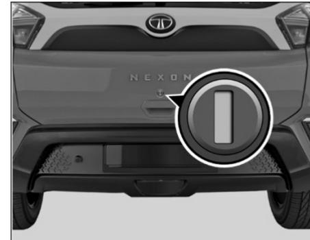
Tail gate opened by using door key, the lock is located on the Tail gate.
