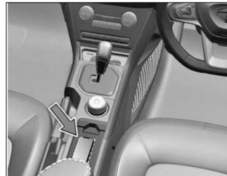
WPC system detects the presence of phone and starts charging as per the Qi standard protocol. The charging status is updated and displayed on the head unit.
