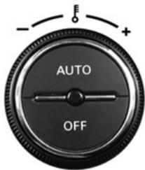
Turning the temperature control knob clockwise increases the temperature of the air. The desired temperature will be increased by steps of 0.5°C. User can select temperature range from 18°C to 30°C. Turning the knob in the anticlockwise direction reduces temperature.
