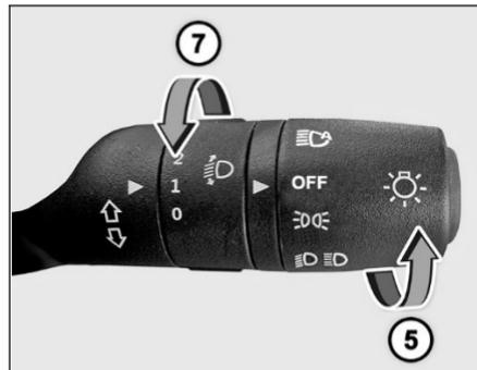
Inner rotary switch on right hand stalk is provided for head lamp leveling. With the inner rotary switch, Head lamp leveling can be done with head lamp in Low Beam and in 'ON' position. Select correct position before start of trip, when the vehicle is stationary. Depending on the number of passengers and luggage in the vehicle headlamp focus may change. This can be adjusted by rotating the knob to one of the three level positions.
