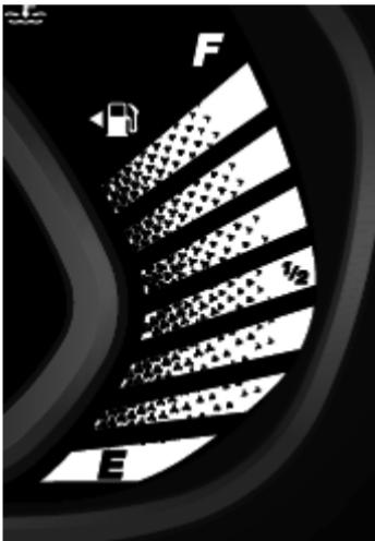
When fuel telltale is moving in the tank nears empty, low fuel warning tell-tale light glows. Fill fuel as soon as possible.
