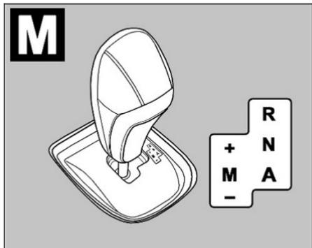
Shift gear lever to left for engaging manual mode. An audio signal indicates when manual mode is engaged. **M** will be indicated in instrument cluster.
