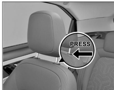
Adjust the head restraint so that it is as close to the head as possible and the center of the head restraint supports the back of the head at eye level. This will reduce the risk of injury to the head and neck in the event of an accident or similar situa-
