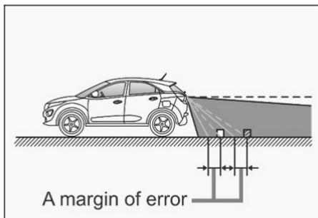
When any part of the vehicle sags due to the number of passengers or the distribution of the load, there is a margin of error between the fixed guide lines on the
