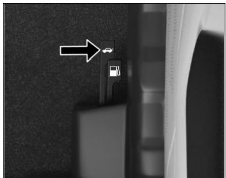
To open the tail gate, pull the lever located at the right hand side below the driver's seat and lift the tail gate.
