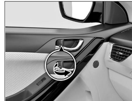
All the doors can also be locked from inside by pressing knob on driver door and independently on other doors respectively.
