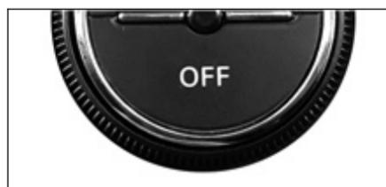
Press the OFF button to switch the system 'OFF'. OFF will be displayed on the infotainment screen.
