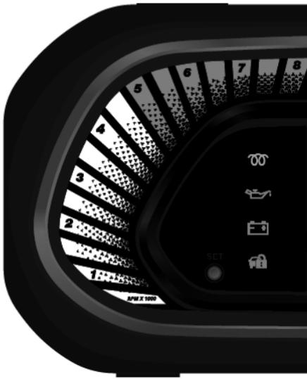
Tachometer indicates engine speed in revolutions per min (rpm).
