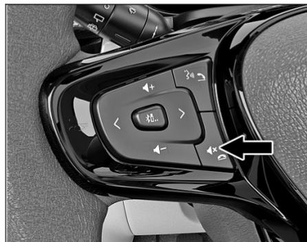
2. Hold the Steering wheel Mute button (long press) for more than 10 secs and then release the button as soon as the display goes blank.
