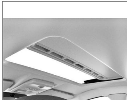
Hold sun shade and move it to rearward direction to open in full position or desired position.
