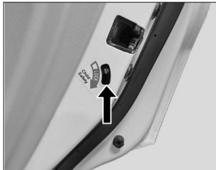
Both the rear doors of the vehicle are provided with a child proof lock. Push the lock lever located on vertical face of the door downward before closing the door. The door which has been closed by activating the child lock cannot be opened from inside, it can be opened only from the outside.
