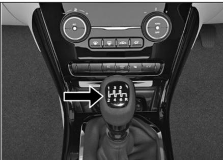
The gearshift pattern is as shown on the gear lever knob. Gear shifting should always be done with the clutch pedal fully pressed.
