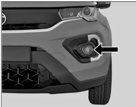
The front fog lamps are located on the front bumper. In poor visibility conditions due to fog, snow or rain, the fog lamps make visibility better and make it easier for other road users to see you. It turns to 'ON' when the fog lamp switch is turned on when the ignition is 'ON' and when the position and parking/ head lamp is 'ON'. An indicator on front fog lamp knob will come on when the front fog light is 'ON'.
