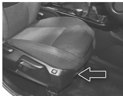
VIN plate below driver seat
