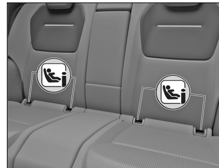
ISOFIX with mounting eyelets
