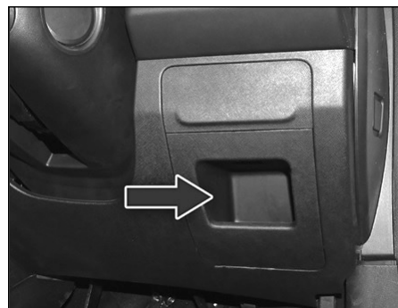
Cabin compartment fuse box
