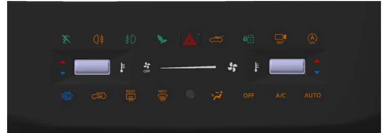
Figure 67 HVAC Control Touch Hard Buttons – Dual Zone
