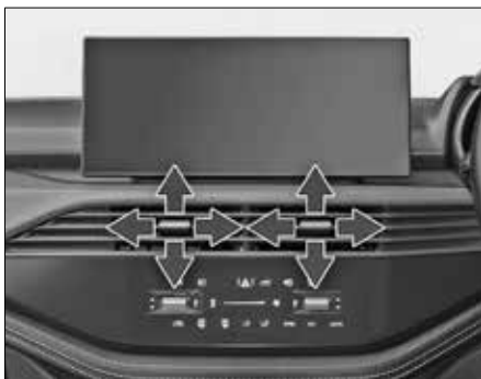
Front Centre Air Vent
