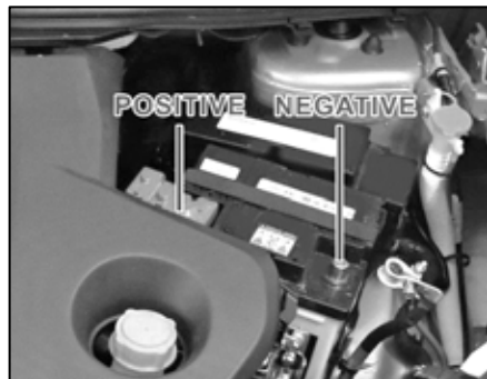
Battery location- Diesel
