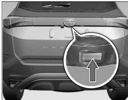
If vehicle is locked and tail gate is closed. Tail gate switch is pressed with valid smart key in the authentication range, Tail gate gets unlatched.
