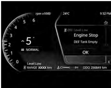
Once the engine is stopped with this message, it will not be possible to restart the engine without filling DEF.
