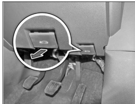
3. Raise the bonnet slightly and with your finger lift (up) the secondary lock lever located under the bonnet center.
