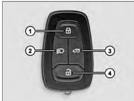
Keep the smart key with user to perform the passive access. It is used for locking, unlocking and starting the vehicle.
