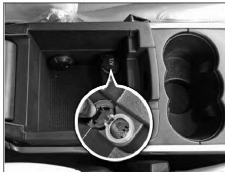
Power socket is available inside the cooled storage box on the center console. The power socket will work when the ignition switch is in the "ACC" or "ON" position. This socket can be used to provide 12V (10A) power for electrical accessories.
