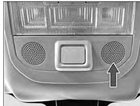
Mics are provided on roof near the roof lamp.
