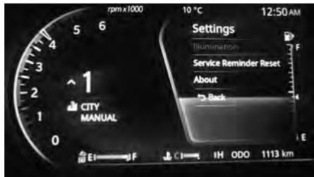
To change the option from unit to service reminder reset by pressing on the RHS of steering switch.
