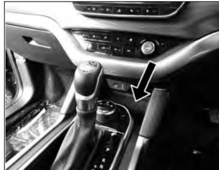
Place for keeping wallet / mobile is provided in front of Gear shifter lever.
