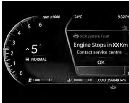
If the vehicle is run without rectifying the SCR system (through TATA MOTORS service centre), warning message will continue with corresponding distance gradually reducing to 0km.
