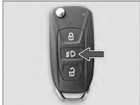
Remote operated Tail gate unlatching can be done through long press (2 sec) approach light button on remote key.
