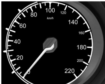
Speedometer indicates the vehicle speed in km/h.
