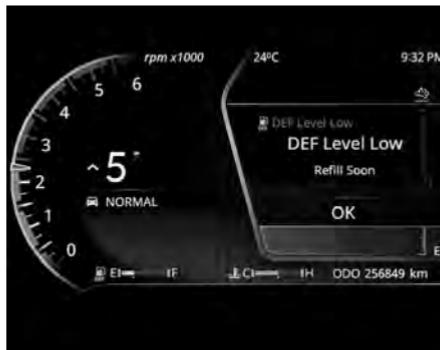
next warning level will be indicated at approximately 600 km before emptying of DEF tank at current DEF consumption rate. “ENGINE STOPS IN 600 KM” message will be indicated at this warning level. This message will continue till DEF tank becomes empty with corresponding distance gradually reducing to 0 km.
