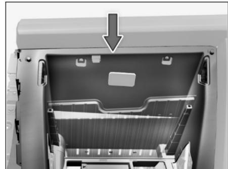
4. Disconnect glove box lamp connection.
