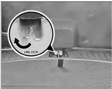
In emergency situation like key or vehicle battery is discharged or electrical malfunctioning, you can unlock the tailgate from inside as per procedure given below:
