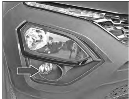
For switching 'ON' the Fog lamps, either the Head Lamp or Parking lamp must be 'ON'.
