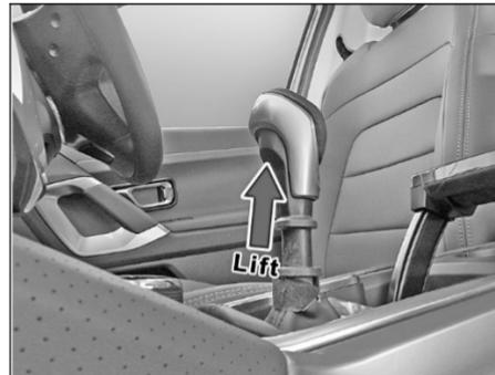
For engaging reverse gear, lift the latch and keeping latch lifted, shift to reverse position.
