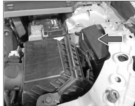
To access the fuse box, follow the procedure as given below:
