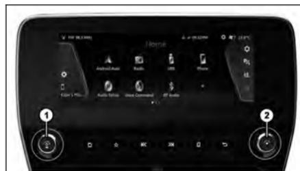
1. Press both the knobs 1 and 2 simultaneously for more than 5 second until system restart.
