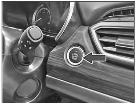
Start/Stop switch is provided on the dashboard towards the right side of steering wheel.
