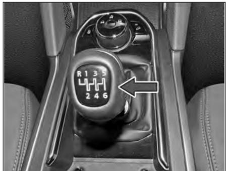
The gearshift pattern is as shown on the gear lever knob. Gear shifting should always be done with clutch pedal pressed.
