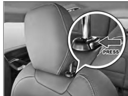
Adjust the head restraint so that it is as close to the head as possible and the center of the head restraint supports the back of the head at eye level. This will reduce the potential for injury to the head and neck in the event of an accident or similar situation.
