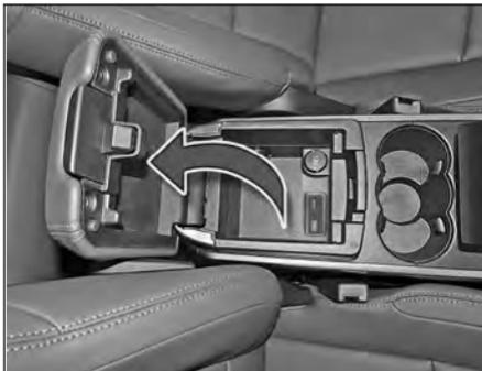
Stowage below front arm rest with chiller is provided on center console between the front passenger seats. It can be used to keep small items.
