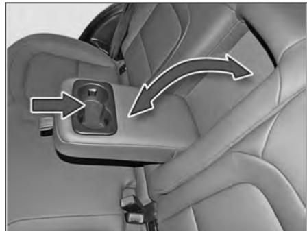
A foldable arm rest has been provided in the rear seat. It also has two cup holders, which can be accessed by opening the cover. When not required, fold the armrest back into the seat.
