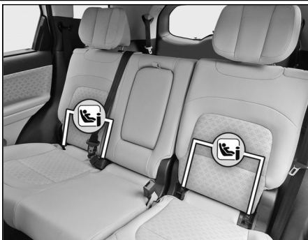
ISOFIX with mounting eyelets
