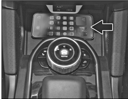
Phone Placement Area
