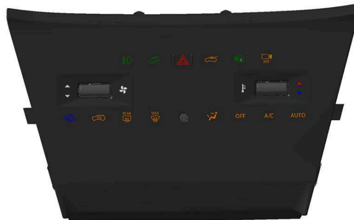
Figure 66 HVAC Control Touch Hard Buttons – Dual Zone
