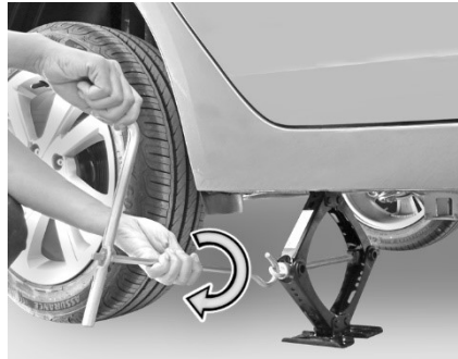
Lifting the front wheel using jack
