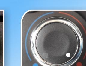
Set blower to max setting and temperature to full hot position.
