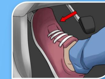
Do not drive your vehicle with foot on clutch pedal.
