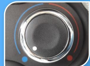
Turn on recirculation mode. Set temperature to desired level.
