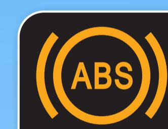
ABS – Antilock braking system provided to avoid skidding of vehicle during braking.
