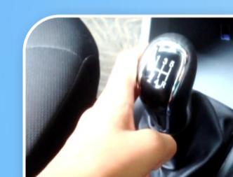
Press clutch fully before shifting gears.
