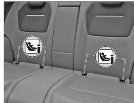
ISOFIX with mounting eyelets
